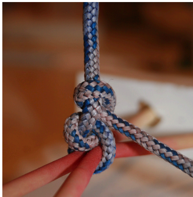
Figure 2 Knot tied under tension producing inadvertent slip knot.
