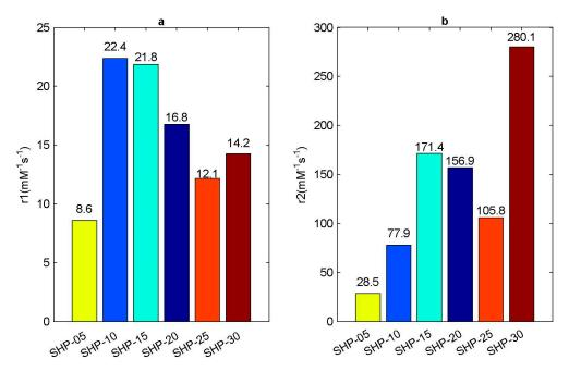
**Figure 5.** Relaxation rate of SHP series magnetic nanoparticle samples. (a)  $r_1$  relaxation rate; (b)  $r_2$  relaxation rate.
