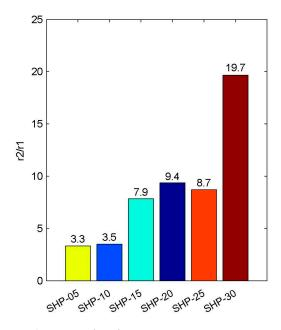
**Figure 6.** The ratio  $r_2/r_1$  of SHP series magnetic nanoparticles.
