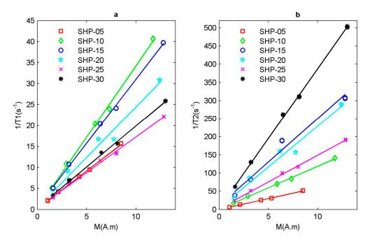
**Figure 7.** Relaxation rate of SHP series magnetic nanoparticle sample. (a) Inverse of longitudinal relaxation time  $1/T_1$  and (b) inverse of transverse relaxation time  $1/T_2$  with respect to the induced magnetization M.
