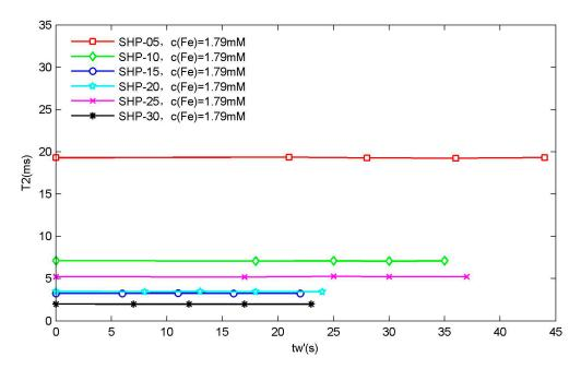
**Figure 3.** Waiting time dependence of  $T_2$  relaxation time. It can be seen that the  $T_2$  relaxation time of magnetic nanoparticle samples with different particle sizes hardly varies with the waiting time  $t'_w$  under the current test conditions.
