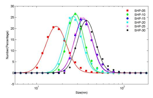
**Figure 2.** Hydrodynamic size distribution of SHP series magnetic nanoparticles. The discrete points are the measured hydrodynamic size distributions, and the solid lines are the fitting curve obtained using lognormal distribution.
