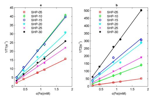
**Figure 4.** Relaxation rate of SHP series magnetic nanoparticle sample. (a) Inverse of longitudinal relaxation time  $1/T_1$  and (b) inverse of transverse relaxation time  $1/T_2$  with respect to Fe ion concentration  $c_{\text{Fe}}$ .
