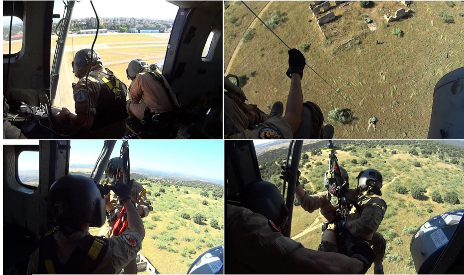
Figure 1. Different moments of the crane rescue maneuver.
