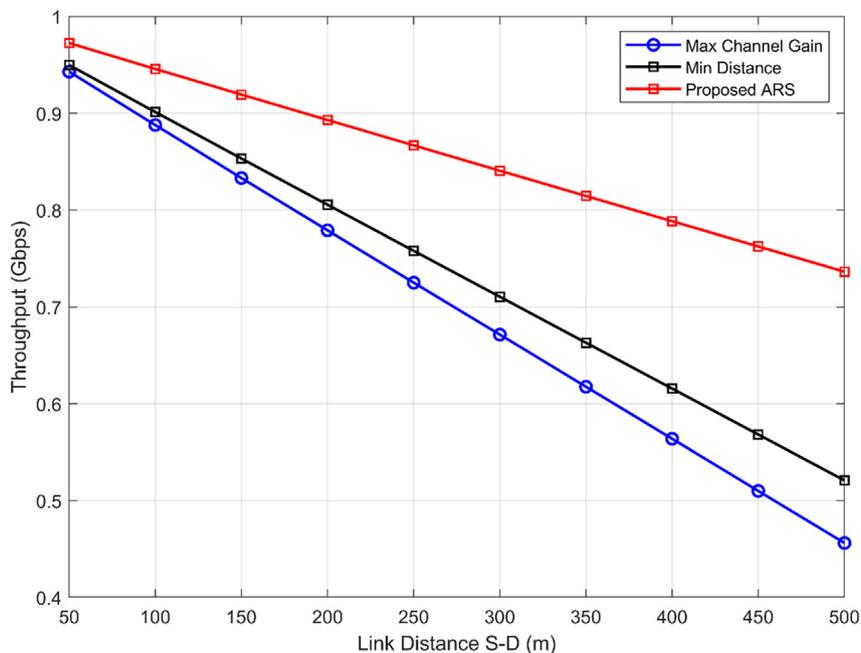
Figure 4. Throughput versus link distance based on the maximum channel gain value, minimum distance, and proposed ARS.
