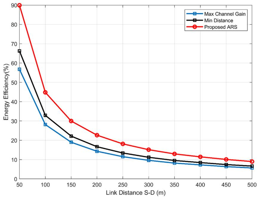
Figure 8. Energy Efficiency versus link distance for the maximum channel gain value, minimum distance, and proposed ARS.
