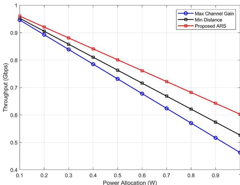
Figure 5. Throughput versus power allocation based on maximum channel gain, minimum distance and proposed ARS.
