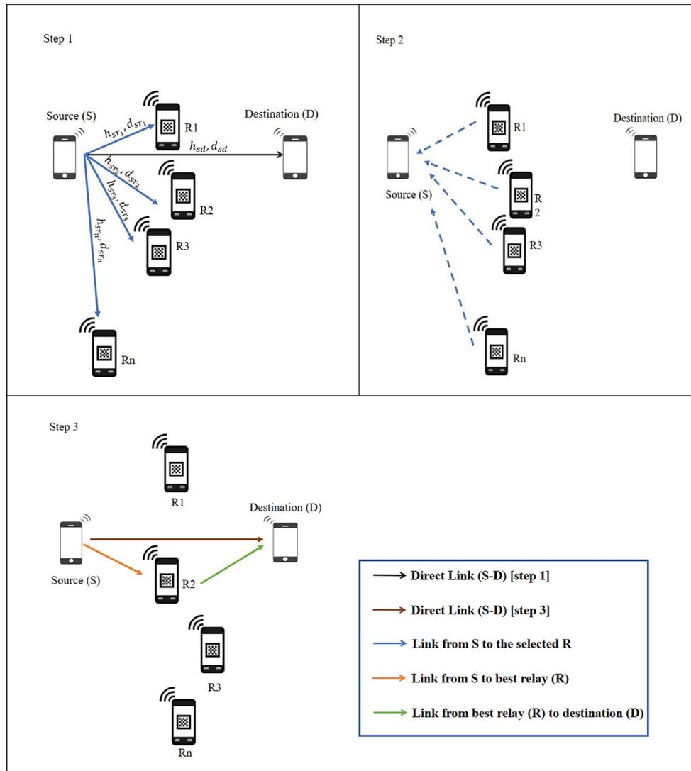
Figure 3. The proposed adaptive relay selection (ARS).
