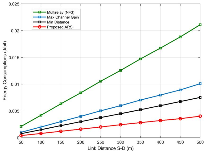
Figure 6. Energy consumption versus link distance for the maximum channel gain value, minimum distance, and proposed ARS.
