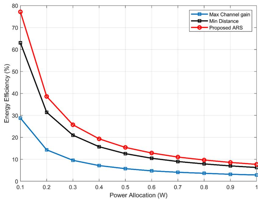
Figure 9. Energy efficiency versus power allocation based on the maximum channel gain value, minimum distance, and proposed ARS.
