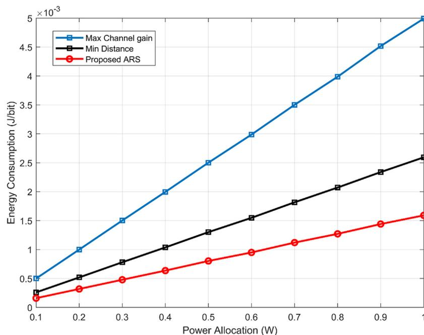
Figure 7. Energy consumption versus power allocation for the maximum channel gain value, minimum distance, and proposed ARS.
