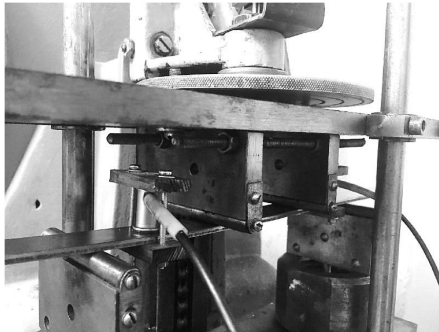
Figure 3. The acoustic emission device for studying bending deformation.
