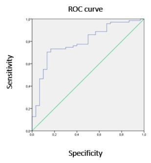
**Figure 1.** Receiver Operating Characteristic (ROC) curve. The blue line represents the union of the cut points of the diagnostic test, the Y axis corresponds to the sensitivity and the X axis to 1-specificity. Both axes include values between 0 and 1 (0% to 100%). The green line represents the reference diagonal or line of non-discrimination, is plotted from point 0,0 to point 1,1.
