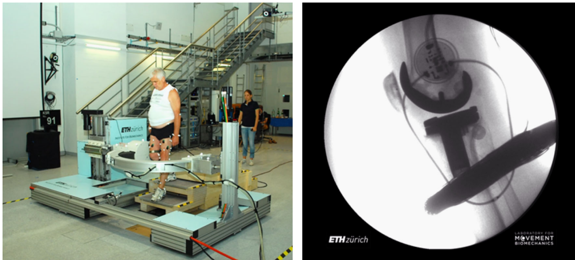
FIGURE 2. The ETH moving fluoroscope was used to capture radiographic images of the knee joints throughout a range of dynamic activities (left). An exemplary fluoroscopic image including the implant component projections is shown on the right. Specific informed consents were acquired from the subjects in order to publish their images.
