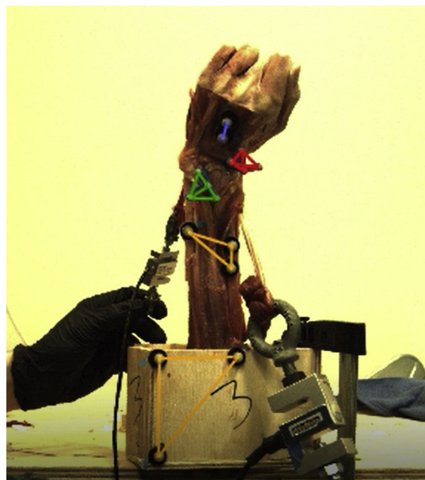
Figure 1. Motion capture setup demonstrating view of wrist with force cells attached to flexor and extensor tendons with overlay of sensors.
