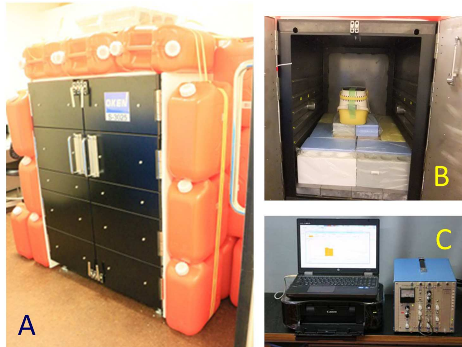
Fig 1. A: Front view of the detection tank of the whole-body counter. The entire surface, including the door, is covered with lead plates. The four vertical outer faces (front, back, left, right) were shielded with water. B: Inside the detection tank. The animal cage can be seen on top of polystyrene blocks. The NaI radiation detectors lie on both sides. C: High-voltage power supply, linear amplifier, multi-channel pulse height analyzer and radioactivity analyzer.
