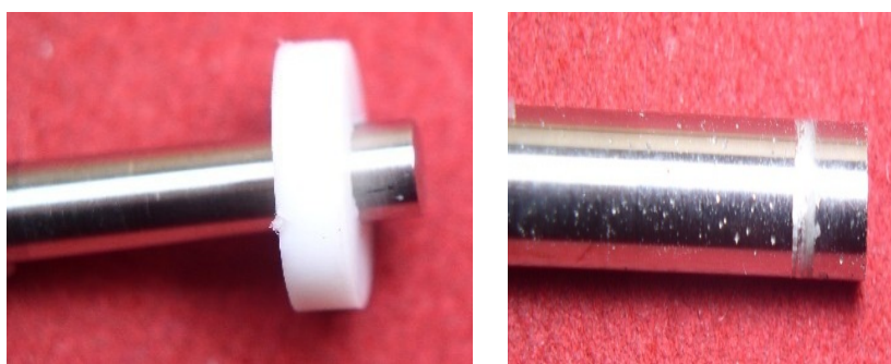
Figure 10. Sample #8 after the crevice-pitting corrosion test.
