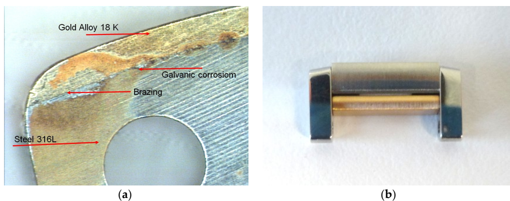
Figure 1. (a) Steel–brazing–gold 18K. (b) Link gold 18K–steel with pins.
