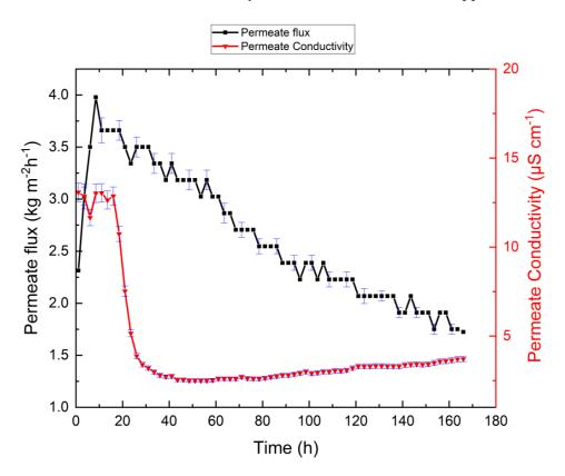
**Figure 5.** Permeate flux and permeate electrical conductivity as functions of time for the synthetic brine feed system with antiscalant. The antiscalant led to higher initial permeate flux compared to the system without antiscalant. Permeate electrical conductivity remained relatively low.
