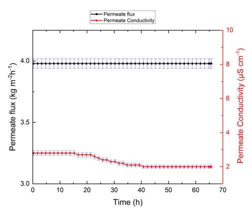
**Figure 2.** Linz tap water VMD test showing permeate flux and permeate electrical conductivity against time. The system exhibited no reduction in permeate flux during the experiment.
