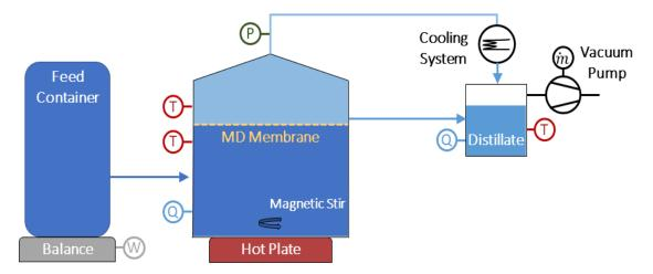
**Figure 1.** Vacuum membrane distillation (VMD) process schematic. The setup consisted of a feed container, a stirred membrane cell, a distillate collection vessel, a feed container, a magnetic stirrer, an external condenser, a balance, and a vacuum pump.
