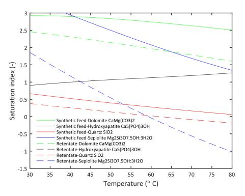
**Figure A9.** Aqueous speciation equilibrium of synthetic RO feed and retentate. Solid lines indicate the saturation indices of secondary precipitated minerals in the synthetic RO feed, while dashed lines indicate the corresponding saturation indices for the retentate. Modeled using PHREEQC software. At low temperatures, silica minerals typically form colloids rather than precipitates. Dolomite requires temperatures above 100 °C for precipitation activation.
