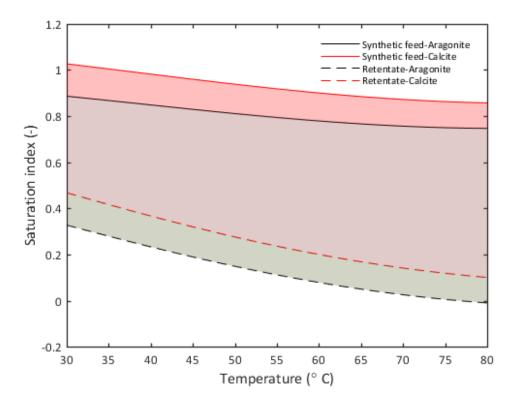
**Figure 4.** Aqueous speciation equilibrium of synthetic RO brine feed without antiscalant and its corresponding retentate. Solid lines indicate the saturation indices of the main mineral precipitates in synthetic RO brine feed without antiscalant, while dashed lines indicate the corresponding saturation indices for the retentate. The shaded area indicates the drop in saturation indices caused by precipitation on the membrane surface. Modeled using PHREEQC software.
