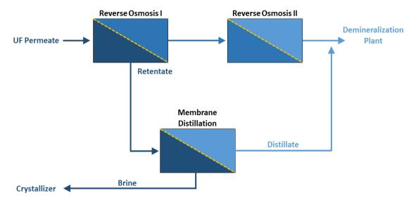
**Figure A1.** Water desalination by an RO + VMD integrated process. The schematic diagram shows the hybrid reverse-osmosis membrane-distillation process for maximizing the system recovery rate and minimizing the environmental impact of brine waste when a VMD unit is added downstream of the RO unit for further recovery.
