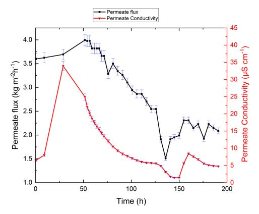
**Figure 3.** Permeate flux and permeate electrical conductivity as functions of time for the synthetic feed system without antiscalant. The permeate flux decreased, which indicates fouling, but permeate electrical conductivity remained at low levels, which indicates the absence of wetting. Feed temperature, permeate temperature, and gauge pressure were kept constant at 75 °C, 21 °C, and -30 mbar during the experiments, respectively.
