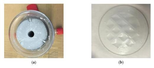
**Figure 6.** After the experiment with synthetic RO brine: (**a**) Membrane module; (**b**) Membrane surface. Salt crystals deposits are visible, which can easily be removed by washing with water.
