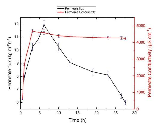
**Figure 7.** Effect of forced (i.e., high-pressure) wetting on system performance. Operation of the process above liquid entry pressure (LEP) led to rapid passage of liquid feed to the permeate side of the membrane, which drastically increased permeate electrical conductivity.
