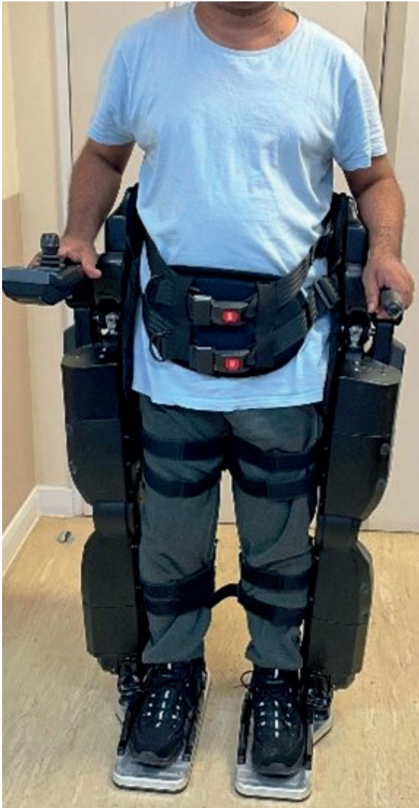
Fig. 3. Individual user inside the Rex robotic Exoskeleton Device from the front. An upright posture, with optimal alignment of the hips, knees and ankles in standing is supported by the device. The user can rest their hands on the bars at the sides. Velcro straps secure the user’s legs, and an abdominal pad across the front is used to assist and support an upright posture. The joystick and controls are visible on one side.
