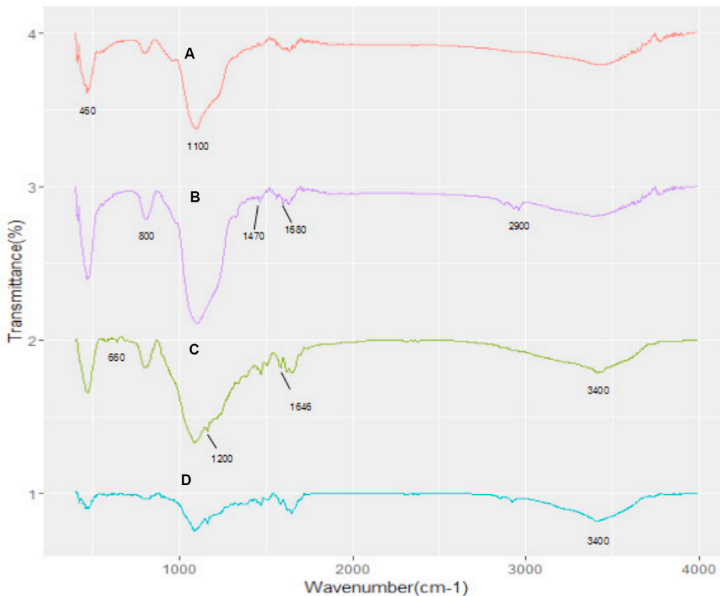
Figure 2: FT-IR spectra of MSN (A), MSN/COOH (B), MSN/COOH/TAT-FITC (C), and MSN/COOH/TAT-FITC/Cit/YSA-BHQ1 (D).
