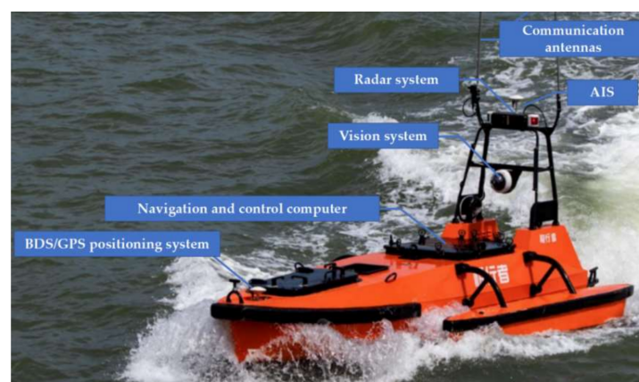
Figure 15. “M80 Polar Walker” USV developed by Yunzhou-Tech Ltd. [29].
