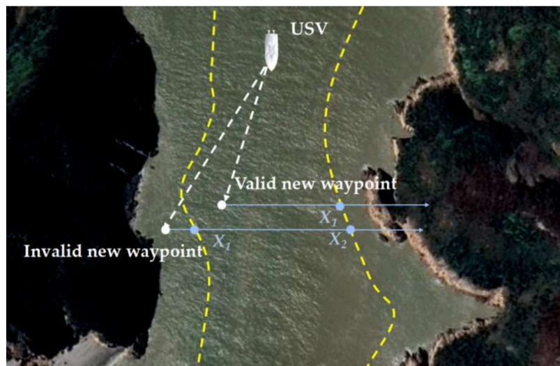
Figure 6. Implementation of terrain constraints using a ray casting algorithm.
