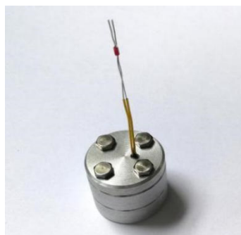
Figure 31. Assembled microexplosive train test tooling.
