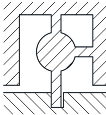
Figure 5. Structure of the shear pin.
