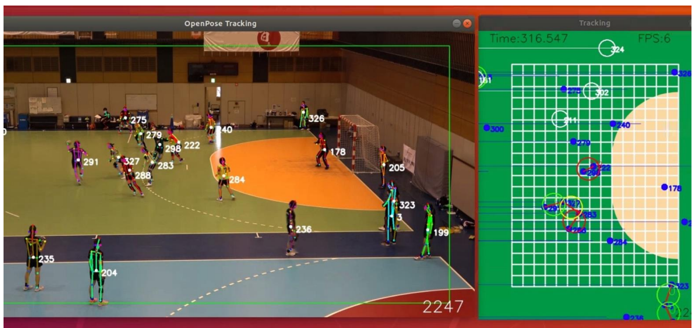
Figure 1. Real-time automated quantitative monitoring of social distancing with a motion image-based AI system, shown on Ubuntu 18.04.5 LST. This system identified participant positions using a function on OpenPose [17]. The distance between the players was calibrated based on known court geometry.
