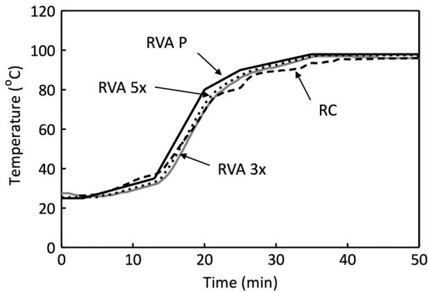
**Fig. 1.** Temperature profile during rice cooking.
