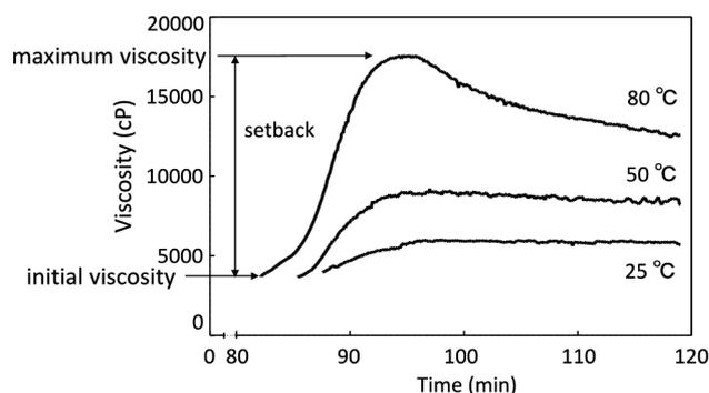
**Fig. 3.** Viscosity profile of cooled samples after high speed shearing at different temperatures.
