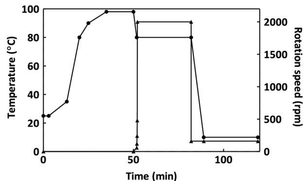
**Fig. 2.** An RVA method profile for continuous protocol from cooking rice to measurement of gel viscosity sheared at 80 °C: temperature (closed circle); rotation speed (closed triangle).
