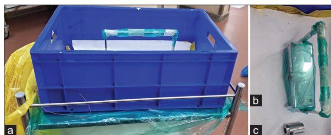
Figure 2: Setup for transportation of radiopharmaceutical from Nuclear Medicine Department (high dose therapy ward) to intervention radiology department; (a) radioactivity transport trolley, (b) syringe carrier, (c) syringe shield
