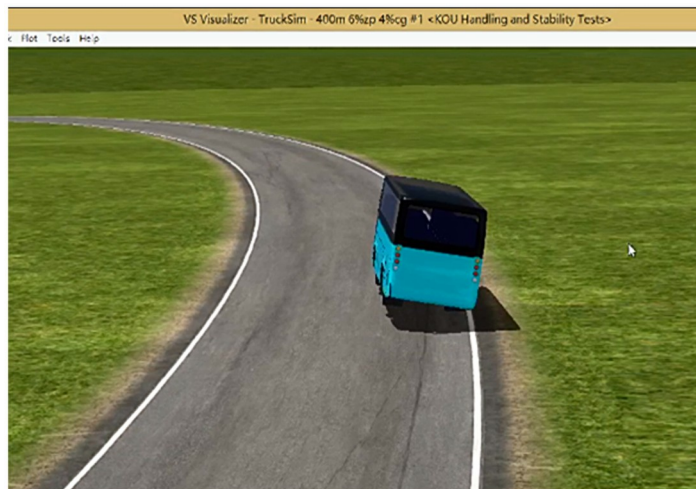
Fig 6. Critical state of large bus sideslip.
