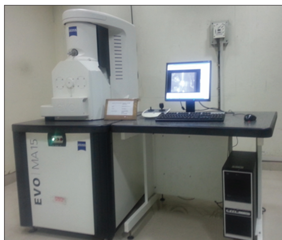
Figure 2: Scanning electron microscope (Carl Zeiss Pvt. Ltd., UK. Model: EVO MA 15)
