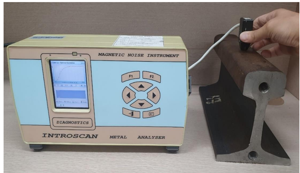
Figure 1. Photograph of the experimental setup for selecting experimental conditions to measure stresses on rails.
