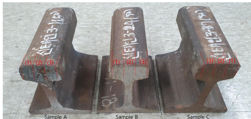
Figure 4. Photograph of three used rail specimens applied in experiments to measure residual stresses by magnetic Barkhausen noise.
