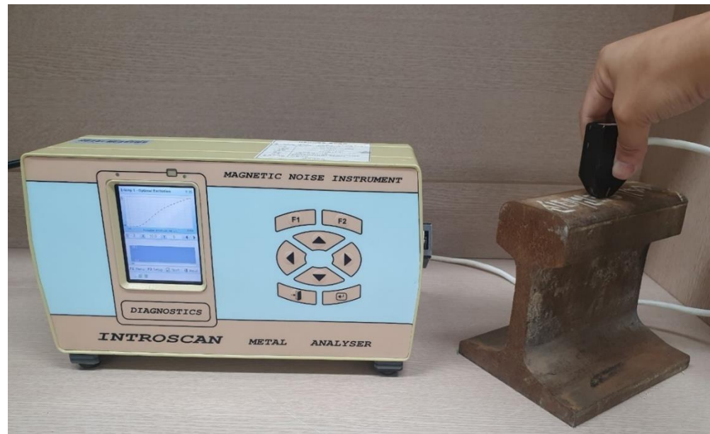
Figure 5. Photograph of the experimental setup for measuring residual stresses in the used rails.
