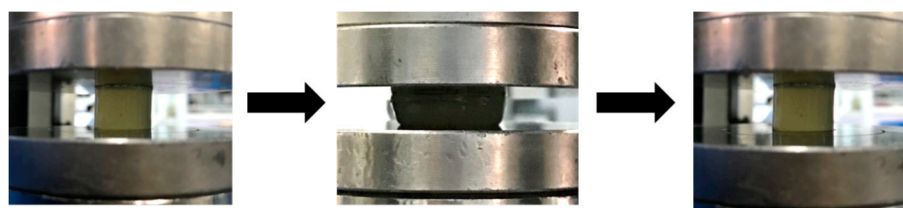
Figure 7. Digital photos of CMC-OSA-DTP hydrogels before and after compressive loading.
