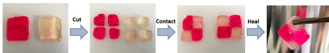
Figure 3. Digital photos of the self-healing process of CMC-OSA-DTP hydrogel pieces (red pieces were stained with rhodamine B for visual discrimination.).
