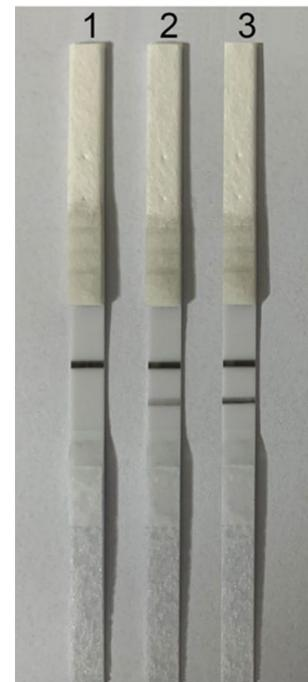
**Fig. 4** p48 protein-labelled CNPs on strips showing different results. Lane 1–3, different ratios (1:4; 1:6; 1:10) of diluted p48 protein-labelled CNPs
