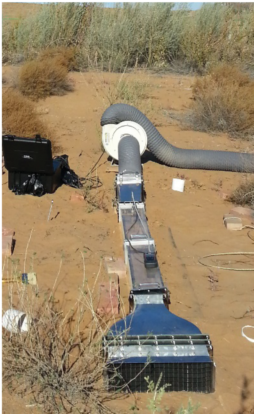
Fig 2. Wind tunnel test in the field.
