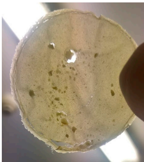
Figure 5. Disc of lemon CytroCell obtained upon mild drying of an aqueous paste.
