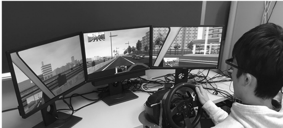
Fig. 2 Experimental layout. The DS used in this study was a modified version of the Honda Safety Navi system, right-hand-drive version (Honda Motor Co., Tokyo, Japan), a DS used for instruction in efficient, safe driving
