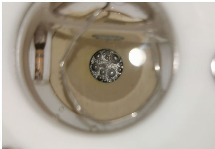
Supplementary Fig. 44 | Photograph of O 2 bubbles covering the surface of a tandem organic IPV-anode during unassisted water-splitting operation.
