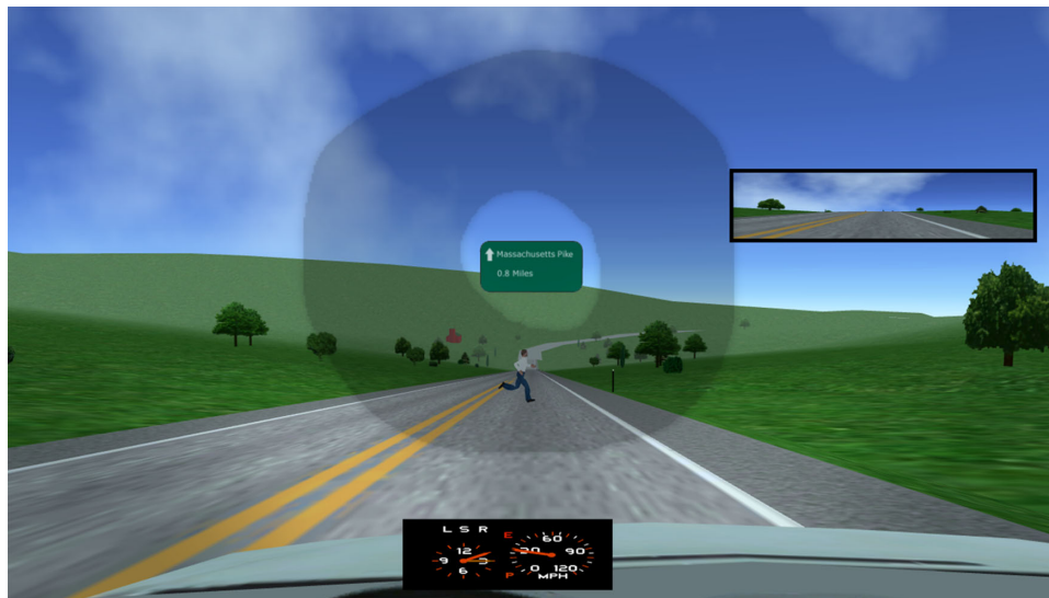
Figure 3. Screen-shot of a sign+pedestrian event, when the vehicle was about 70 meters from the sign and 35 meters from the pedestrian. The pedestrian was programmed to appear, run across the road ahead of the driver for about 1 second, and disappear, all while the participant was reading the sign through the bioptic. The pedestrian was within the ring scotoma area in the monocular visual field (shown by grey shading for illustration purposes only). The small area around the sign, without shading, is the field of view through the telescope. That field of view when magnified covers the full extent of the ring scotoma. Only the central monitor of the simulator is shown; the inset on upper right is the rearview mirror.
