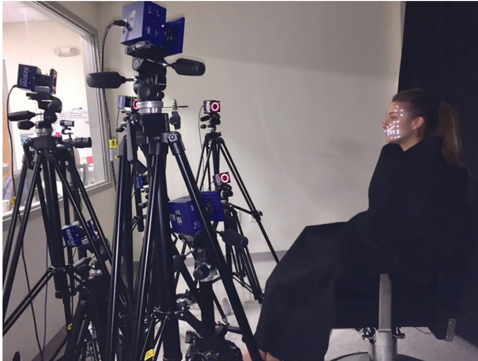
Fig. 1. Motion Analysis System used to record 3D facial landmark movements of each participant during different facial movements or animations.
