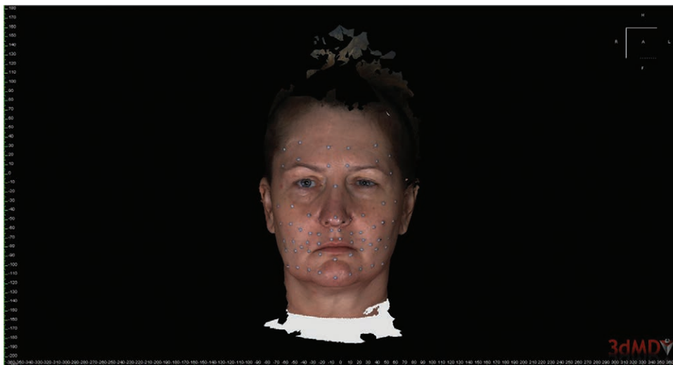
Fig. 2. Three-millimeter, hemispherical, retro-reflective landmarks secured to 64 specific sites on the faces of patients with facial paralysis and the control participants.
