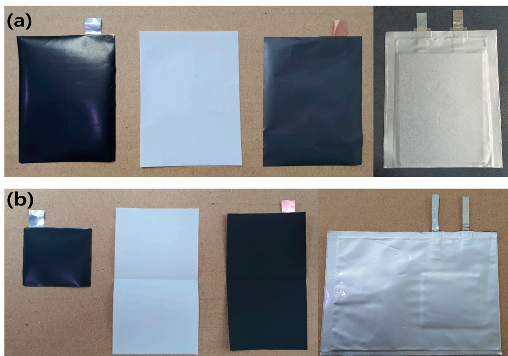
Figure 1. Photographs of the cathode, separator, and anode components (left) and the assembled cells (right) for the (a) PFCs and (b) SLPCs.
