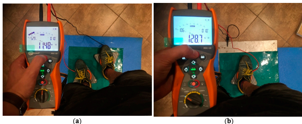
Figure 10. (a) Point-to-point and (b) vertical resistance measurement.
