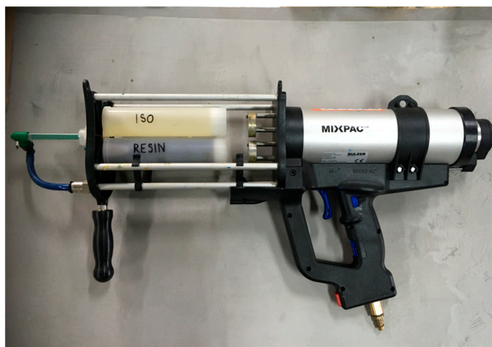
Figure 9. Pneumatic dispenser equipped with a cartridge and static mixer.
