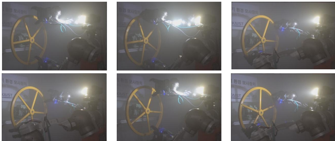
Figure 13. The snapshot of the robot turning the valve in dense fog condition.
