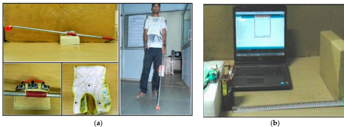
Figure 18. (a) The prototype of the device; (b) Detection process of the obstacle from 5 cm to 150 cm [38].
