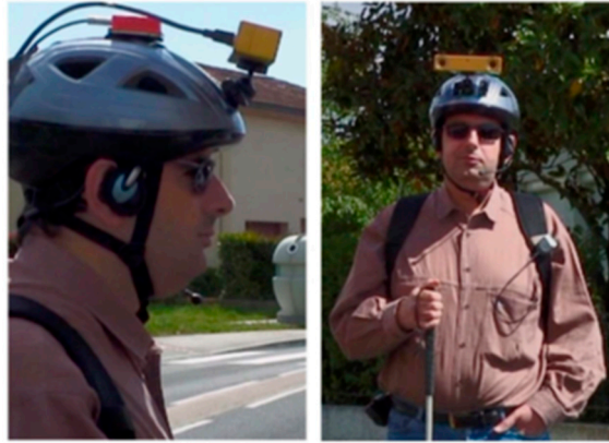
Figure 6. An assistive device for blind people based on a map matching approach and artificial vision [22].
