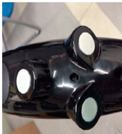
Figure 33. Replacement of three ultrasonic sensors on the cane [54].
