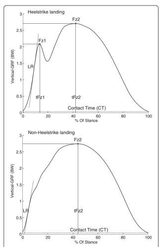
Figure 1 Outcome measures in a typical vertical groundreaction force (GRF) curve for a heelstrike runner and a nonheelstrike runner. Figure is created from personal data.
