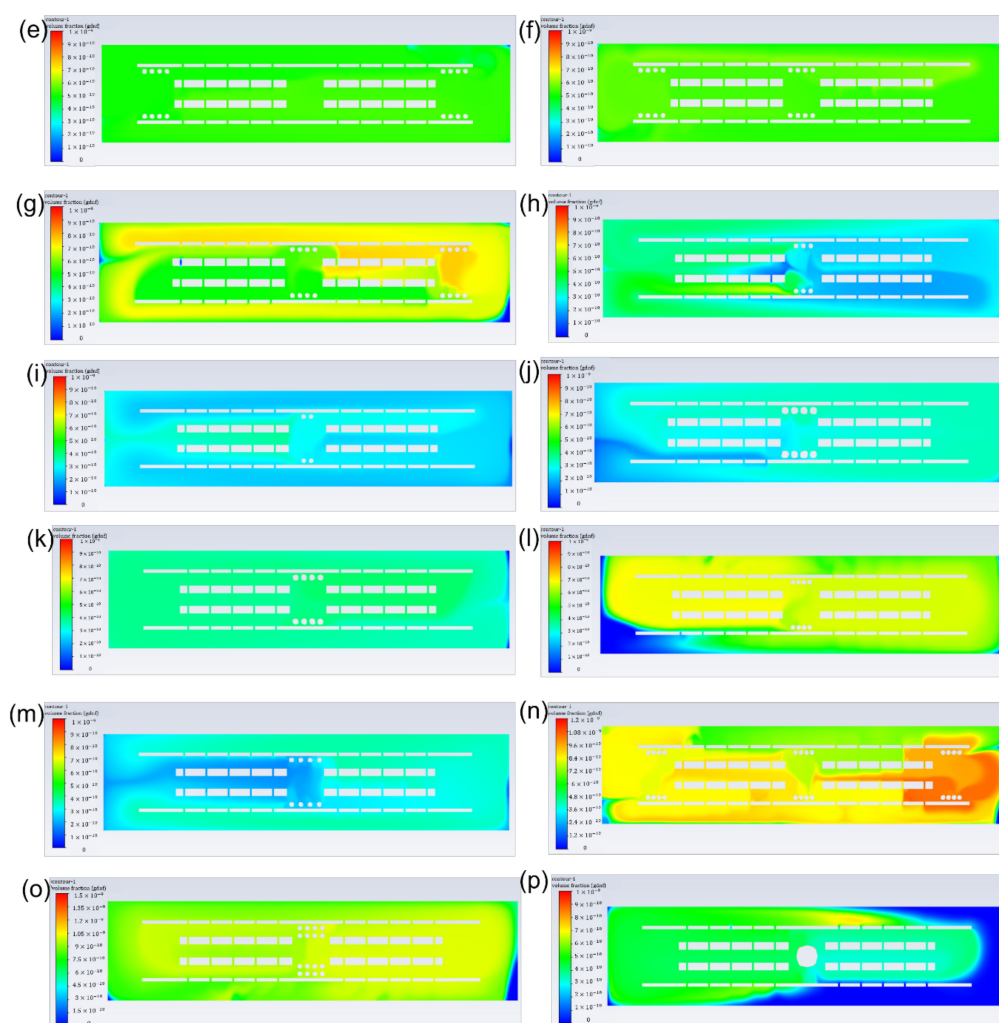
Figure 4. GDNF distribution of different drug release systems under the assumption of constant simulation time. (a) Single-layer microsphere system (microsphere features: quantity: 8; diameter: 0.1 mm; adjacent distance: 0.2 mm; position: middle); (b) single-layer microsphere system (microsphere features: quantity: 8; diameter: 0.1 mm; adjacent distance: 0.2 mm; position: front); (c) single-layer microsphere system (microsphere features: quantity: 8; diameter: 0.1 mm; adjacent distance: 0.2 mm; position: back); (d) single-layer microsphere system (microsphere features: quantity: 24; diameter: 0.1 mm; adjacent distance: 0.2 mm; position: front+middle+back); (e) single-layer microsphere system (microsphere features: quantity: 16; diameter: 0.1 mm; adjacent distance: 0.2 mm; position: front+back); (f) single-layer microsphere system (microsphere features: quantity: 16; diameter: 0.1 mm; adjacent distance: 0.2 mm; position: front+middle); (g) single-layer microsphere system (microsphere features: quantity: 16; diameter: 0.1 mm; adjacent distance: 0.2 mm; position: middle+back); (h) single-layer microsphere system (microsphere features: quantity: 6; diameter: 0.1 mm; adjacent distance: 0.2 mm; position: middle); (i) single-layer microsphere system (microsphere features: quantity: 4; diameter: 0.1 mm; adjacent distance: 0.2 mm; position: middle); (j) single-layer microsphere system (microsphere features: quantity: 8; diameter: 0.15 mm; adjacent distance: 0.2 mm; position: middle); (k) single-layer microsphere system (microsphere features: quantity: 8; diameter: 0.125 mm; adjacent distance: 0.2 mm; position: middle); (l) single-layer microsphere system (microsphere features: quantity: 8; diameter: 0.1 mm; adjacent distance: 0.15 mm; position: middle); (m) single-layer microsphere system (microsphere features: quantity: 8; diameter: 0.1 mm; adjacent distance: 0.25 mm; position: middle); (n) single-layer microsphere system (microsphere features: quantity: 8; diameter: 0.1 mm; adjacent distance: 0.15 mm; position: front+middle+back); (o) double-layer microsphere system; (p) bulk hydrogel system.
