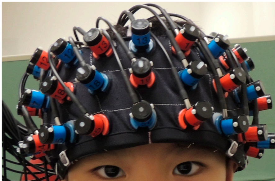
Figure 2. The 3 \times 11 montage of the functional near-infrared spectroscopy (fNIRS) system: (a) 33 optodes and 52 channels (CH) arrangement; (b) placement on head.
