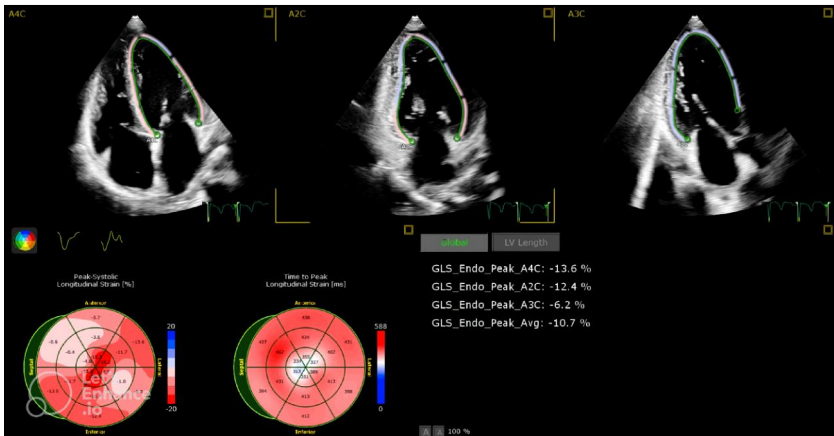
Figure 4 Assessing LVGLS with STE: a comprehensive view from four-chamber, three-chamber, and two-chamber views. This image captures LVGLS analysis using Philips vendor's advanced speckle tracking technology in an ESRD patient before KTx. The speckle tracking software precisely analyses myocardial tissue movement based on speckle patterns within the cardiac images obtained from four-chamber, three-chamber, and two-chamber views. By tracking these speckles throughout the cardiac cycle, it quantifies LV strain during systole and diastole. The LV strain values are expressed as negative percentages (%) in figure.
