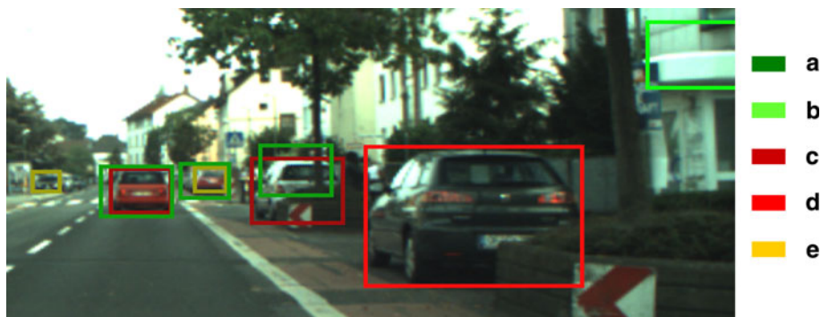
Fig. 15 Example of single-image performance evaluation. a Hypothesis matching an annotation (true-positive case) b hypothesis not matching any annotation in the current image (false-positive case) c annotation matched by one or more hypotheses d annotation not matched by any hypothesis (false-negative case) e annotation that is not considered due to size constraints, see text. Such annotations do not constitute a false-negative case when matched by a hypothesis, but neither a true-positive case otherwise
