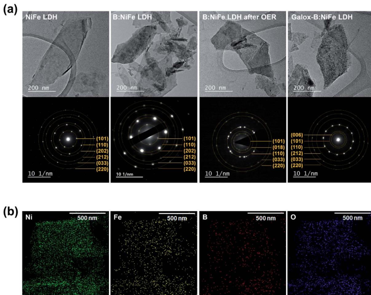
Fig. 2 Further morphological characterization of B:NiFe LDH before and after galvanostatic oxidation. (a) Transmission Electron Microscopy (TEM) analysis (top of each row) and selected area electron diffraction (SAED) pattern (bottom of each row) of the NiFe LDH-based electrocatalyst under each condition. (b) EDS mapping of TEM images of the B:NiFe LDH chemical composition.
