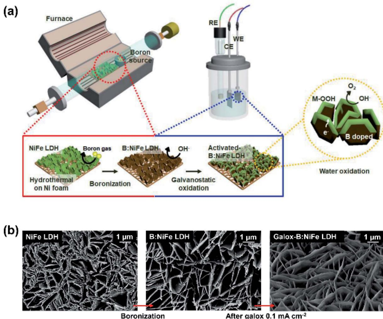
Fig. 1 Summary of the fabrication scheme and structural and morphological characterization of galvanostatically oxidized nickel–iron layered double hydroxide (NiFe LDH) with boron doping. (a) Schematic illustration of the synthesis of galvanostatically oxidized boron-doped NiFe LDH (galox-B:NiFe LDH) through gas–solid boronization in a furnace and electrochemical oxidation. (b) Field-emission scanning electron microscopy (FE-SEM) images of the NiFe LDH-based electrocatalyst under each condition.
