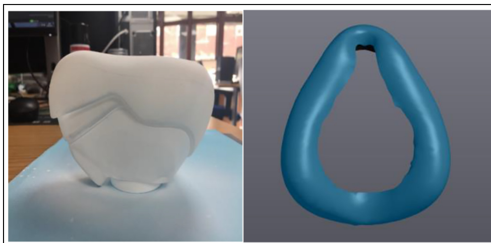
Figure 7. Painted Full-faced interface model (left) and 3D model construction of Full-faced interface cushion (right).
