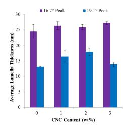
**Figure 5.** Average crystal lamella thickness of the two dominant diffraction peaks, 16.7° and 19.1°, for the CNC/PLA films as a function of CNC content.
