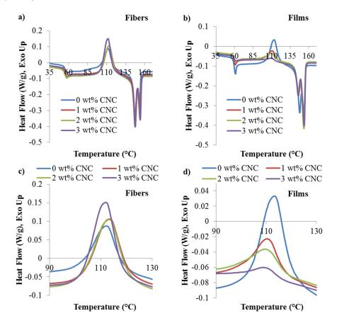
**Figure 2.** Non-isothermal initial heating thermograms of CNC/PLA (**a**) fibers; (**b**) films; (**c**) fiber cold crystallization peaks; and (**d**) film cold crystallization peaks.
