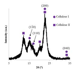
Figure 4. Diffraction pattern of a CNC mat with cellulose I and cellulose II primary diffraction peaks indicated.
