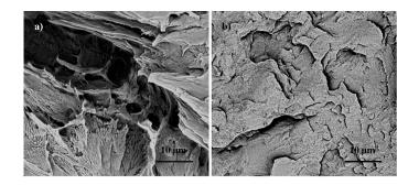
**Figure 1.** Representative scanning electron micrographs images of cryo-fracture surfaces for (**a**) 0 wt % cellulose nanocrystals/poly lactic acid composites (CNC/PLA) and (**b**) 3 wt % CNC/PLA composites.
