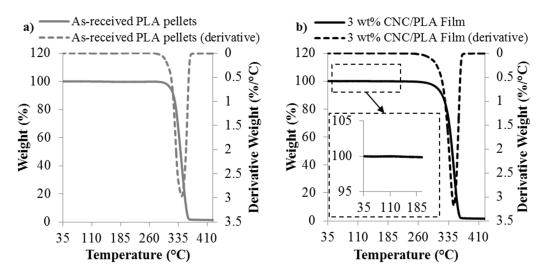
**Figure 8.** Representative results of the thermogravimetric analysis (TGA) of the (**a**) as-received PLA pellets and (**b**) 3 wt % CNC/PLA film.
