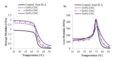
Figure 6. (a) Storage modulus and (b) loss modulus of the CNC/PLA films as a function of CNC content.
