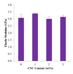
Figure 7. Elastic modulus of CNC/PLA films as a function of CNC content.
