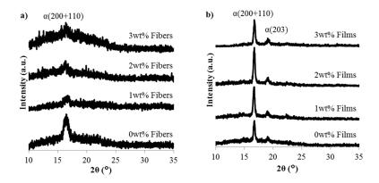
**Figure 3.** Diffraction patterns obtained for the CNC/PLA (**a**) fibers and (**b**) films as a function of CNC content.
