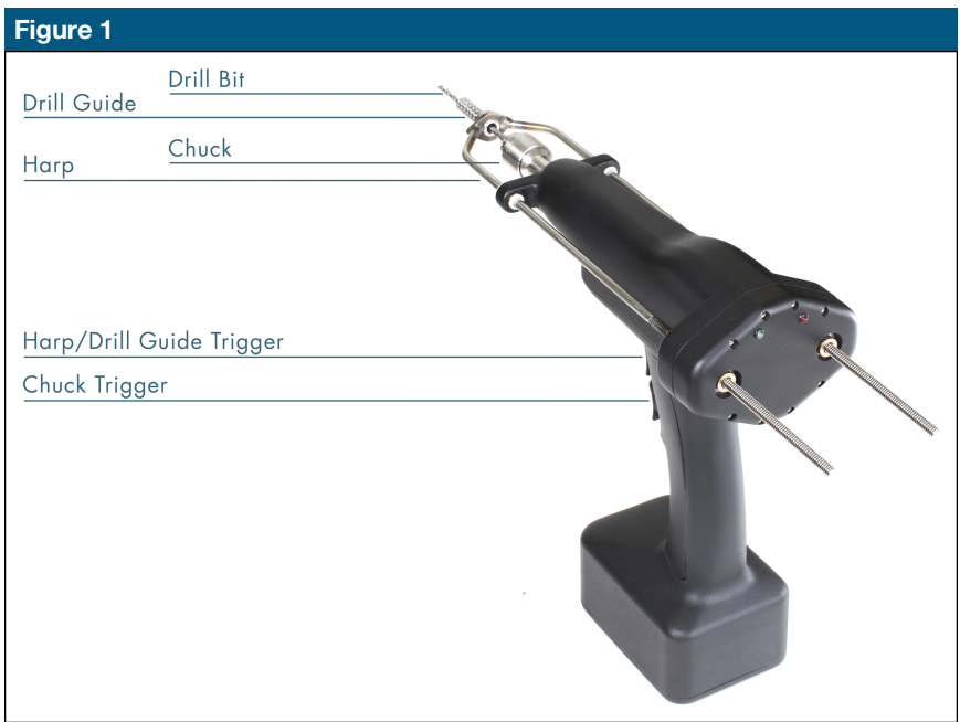
Photograph of the dual motor drill. Collectively, the drill functions like a handheld drill press. Depression of the chuck trigger engages the first motor to spin the chuck similar to any standard orthopaedic drill. Depression of the harp and drill guide trigger engages the second motor to move the harp and drill guide parallel to the axis of the drill bit. During drilling, the drill bit moves forward at a controlled rate, whereas the harp and drill guide remain fixed. The harp and drill guide function as a variable depth stop, whereas the drill guide functions as a tissue protector.
