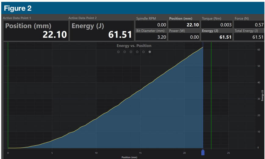
Example of visual monitor demonstrating the energy plot with energy (y-axis) in joules and position (x-axis) in millimeters for a 22-mm hole drilled in a 20-pcf block. When the drill bit reaches the desired depth (position), the operator stops drilling by letting go of the triggers. The total energy can be recorded for any given depth (position) on the plot.
