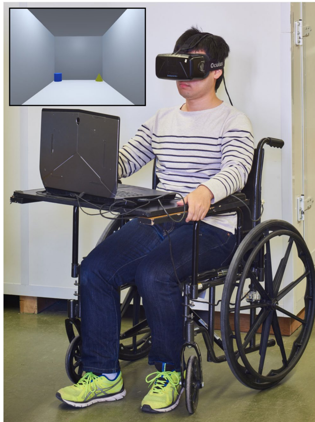
Figure 2. The VRNChair including laptop and HMD. The inset photo gives an example of the virtual room as viewed through the HMD. Physical movement of the VRNChair translated to movement within the virtual room. Choices were made by pressing a button attached to the participant's right finger (not shown).
