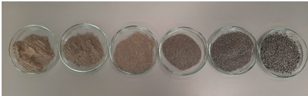
Figure 1. Grain fractions of concrete aggregate, from the smallest from the left: <0.063\text{ mm} ; 0.063\text{--}0.125\text{ mm} ; 0.125\text{--}0.25\text{ mm} ; 0.25\text{--}0.50\text{ mm} ; 0.5\text{--}1.0\text{ mm} ; 1.0\text{--}2.0\text{ mm} .
