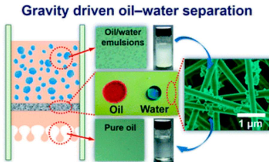
**Figure 12.** Gravity-driven separation of surfactant-stabilized water-in-oil microemulsions by fluorinated polybenzoxazine (F-PBZ) coated functionalized silica nanofibrous membranes (F-SNF/ $\text{Al}_2\text{O}_3$ ). Reproduced from [145] with permission from The Royal Society of Chemistry.
