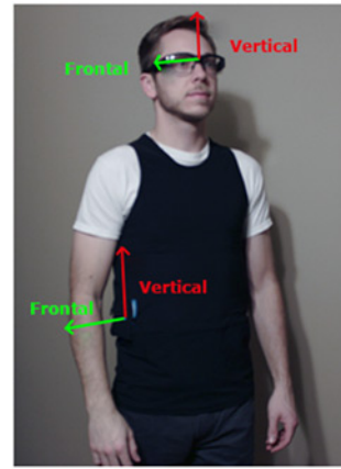
Fig. 2 Placement of sensors on the subject and alignment of axes between sensors
