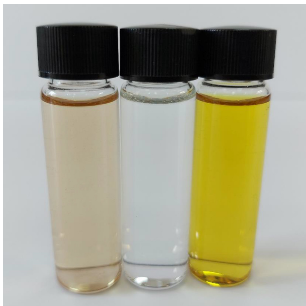
Fig. 2. Strong color change upon mixing TCNE (far left; pale brown) with AZM (middle; colorless) to produce the CT complex (far right; intense yellow) in the \text{CH}_3\text{CN} solvent.
