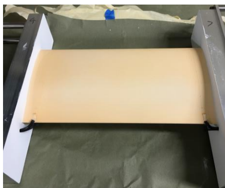
Figure 1. HSNLF(1)-0213 airfoil coated with TSP/CNT.
