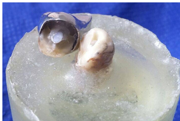
Fig. 4 Photograph representing an example of a favorable type of failure with detachment of the post and core system that could be repaired.
