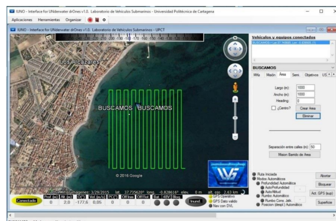
Figure 5. Graphical User Interface of IUNO software, showing exploration routes within a 1 km × 1 km box given by the four geographical coordinates (UTM) P1 (30T 690 4180), P2 (30T 690 4179), P7 (30T 691 4180) and P8 (30T 691 4179).
